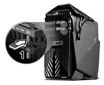
When the disk tray slides open, place the disk gently on the tray. Make sure that the label or title side of the disk is facing upward. When holding a disk, hold it by the edges to avoid leaving smudges or fingerprints.
